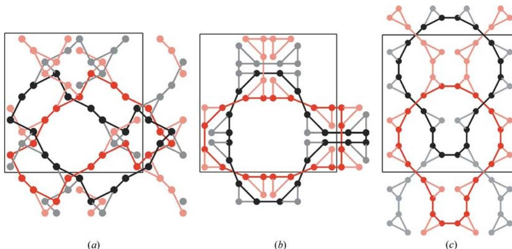
**Figure 1** Interpenetrating sphere packings belonging to types (a) *c*[3/3/*c*1]<sup>2</sup><sub>I</sub>, (b) *c*[3/3/*c*1]<sup>2</sup><sub>II</sub> and (c) *c*[3/3/*c*1]<sup>2</sup><sub>III</sub>. Interpenetration patterns *c-e*, *c-f* and *c-a*, respectively.
